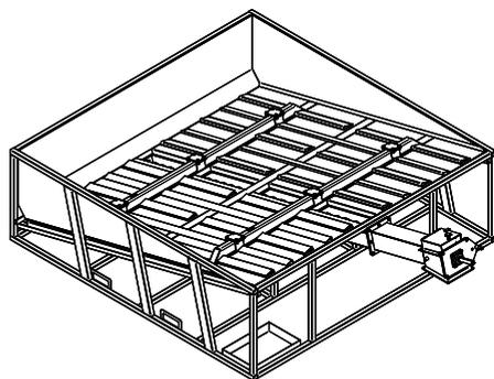
**Note! The bottom-edge of the side walls built on-site must be level with inner surface of the walking floor walls.**
