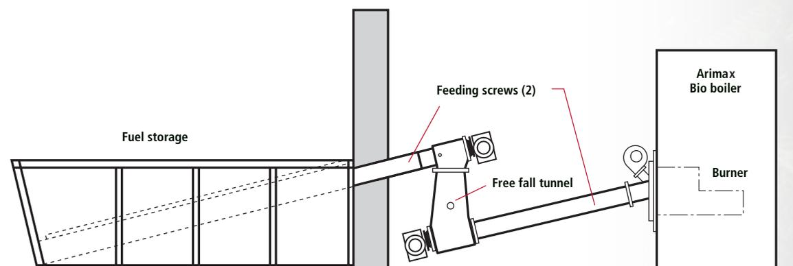
The recommended maximum length of the screws is 5 m. The minimum lengths of different systems can be found in the reference drawings in the brochure (p. 34–45).
